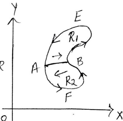
say  $R_1$  and  $R_2$  as shown in the figure by drawing a line AB. In this case we apply the theorem to each sub region  $R_1$  and  $R_2$  separately and then add the results.
